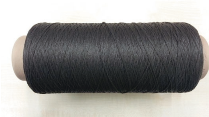
Fig. 8 BCF bobbin with 100 % physical recycled material (Source Gneuss GmbH)
