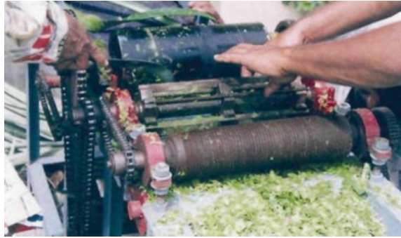
Fig. 15 Scrapping machine of pine leaves [50]
